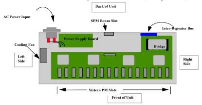
Figure 3.10b: Magnum 8000X, Top View with Chassis Cover Off
